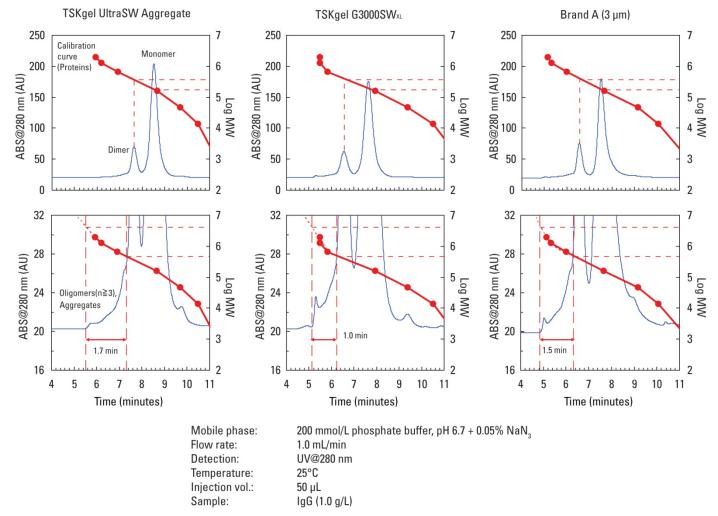
The TSKgel UltraSW Aggregate possesses a wider separation window for IgG oligomers and aggregates with high MW (5x10<sup>5</sup>~5x10<sup>6</sup> Da) than other SEC columns.
